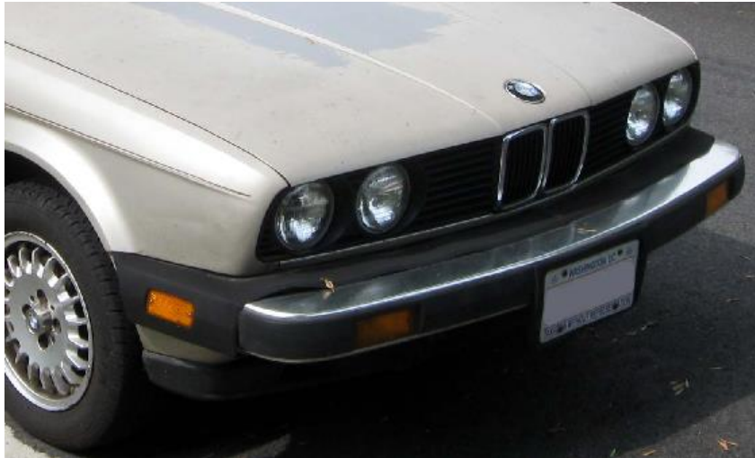
BMW 325e sedan (produced for the North American market in 1984–1987) with elongated front and rear aluminium bumpers
