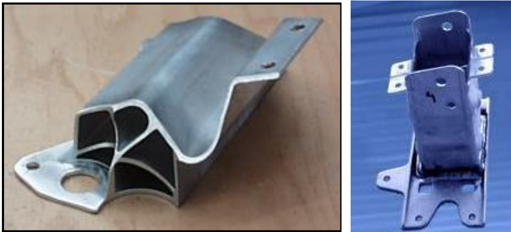
Crash boxes made from extruded aluminium profiles designed for transverse (left) and axial folding (right)
