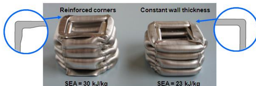
Reinforced corners increase the specific energy absorption capacity (SEA) of aluminium extrusions
