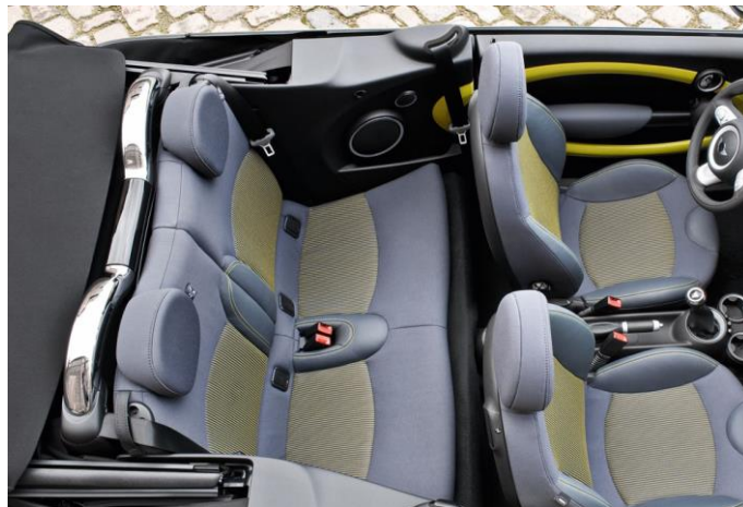
Roll-over protection system of the Mini cabriolet, the one-piece aluminium bar (Photo: Mini)
