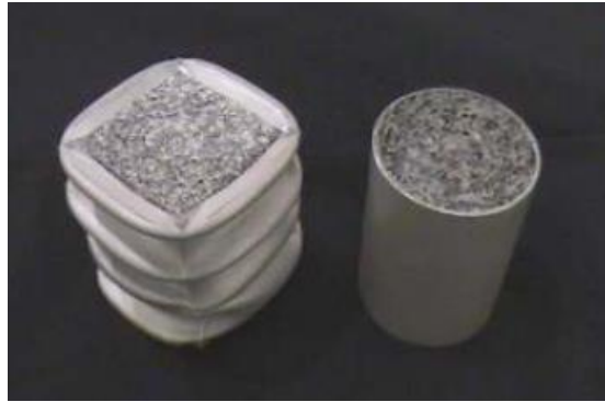
Extruded profiles filled with aluminium foam for crash boxes
