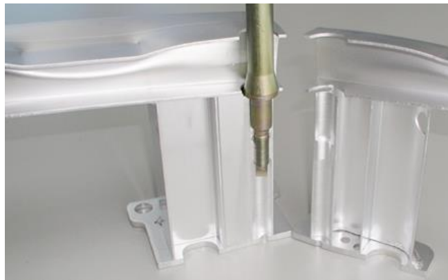
Integration of the towing function into a crash box
